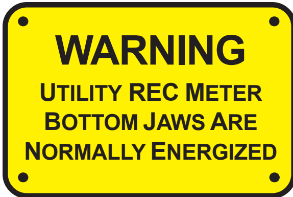
Tag 1. Install On Meter Box
