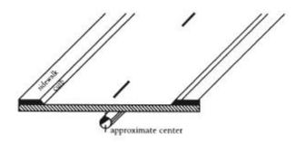
As an alternative, or in addition to, marks can be placed on either side of the facility to define the "Hand Dig Area". The "Hand Dig Area" is defined as the width of the facility itself plus the tolerance zone of 30" on either side of the facility.
