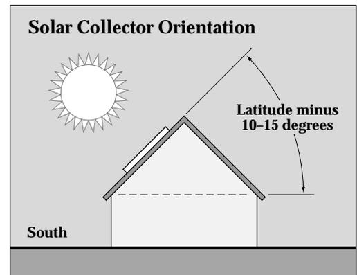
**For heating primarily in the summer, the tilt of a solar collector should equal the latitude where the pool is located minus 10 to 15 degrees.**
