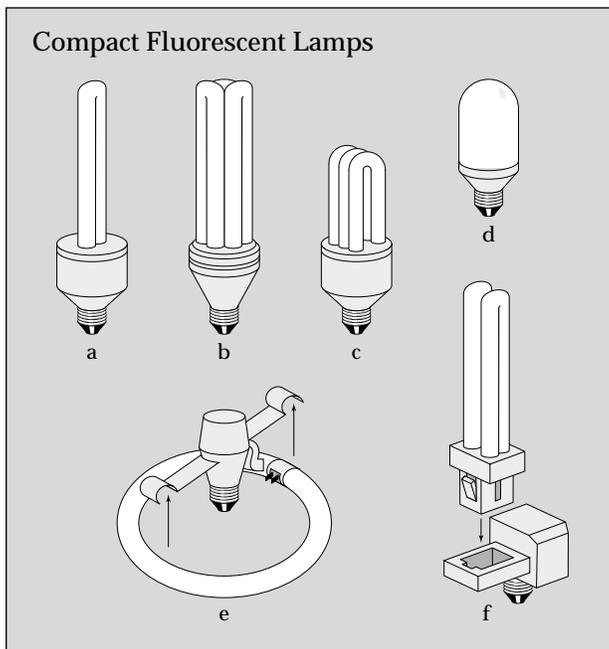
Compact fluorescent lamps (CFLs) come in a variety of sizes and shapes including (a) twin-tube integral, (b and c) triple-tube integral, (d) integral model with casing that reduces glare, (e) modular circline and ballast, and (f) modular quad-tube and ballast. CFLs can be installed in regular incandescent fixtures, and they consume less than one-third as much electricity as incandescent lamps do.
