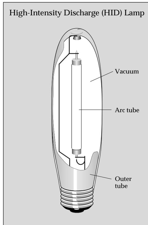
In a high-intensity discharge lamp, electricity arcs between two electrodes, creating an intensely bright light. Mercury, sodium, or metal halide gases act as the conductor.
