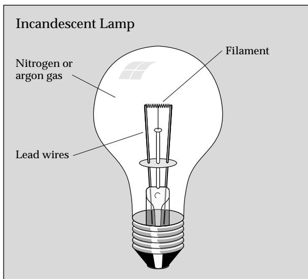
The incandescent lamp is the oldest and most common type of lamp. Light is emitted when electricity flows through—and heats—a tungsten filament.
