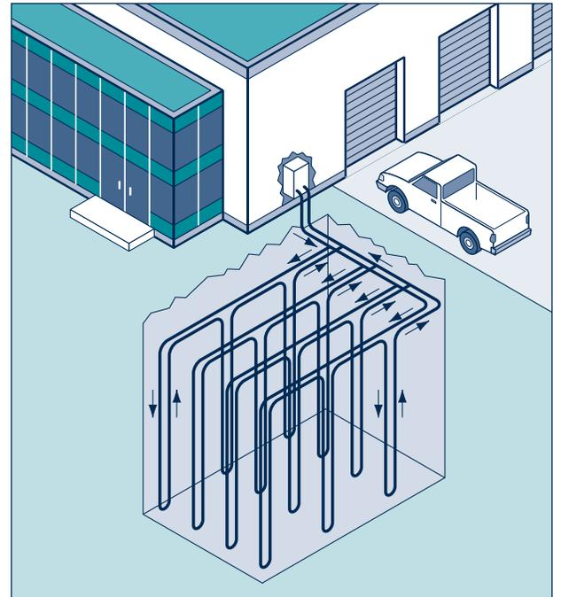
Geothermal heat pumps use the stable temperature of the ground (vertical boreholes typically are 100 to 400 feet deep) as a heat source to warm buildings in winter and as a heat sink to cool them in summer.
