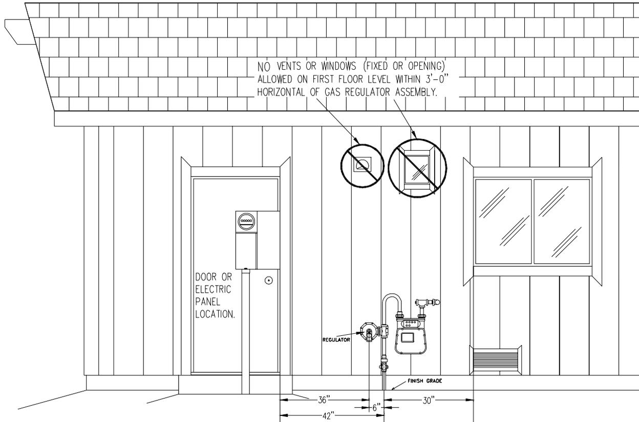
IN APPLYING DIMENSIONS AS SPECIFIED, THE REGULATOR VENT SHALL BE 36" FROM ANY OPENING INTO A BUILDING.
