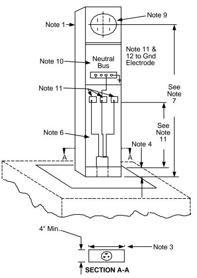
200 Amps, 240 Volts Maximum, Single or Double Meter Post
