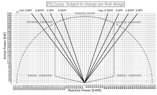
\* Operation area will be curtailed by input DC voltage, output AC voltage and temperature condition.
