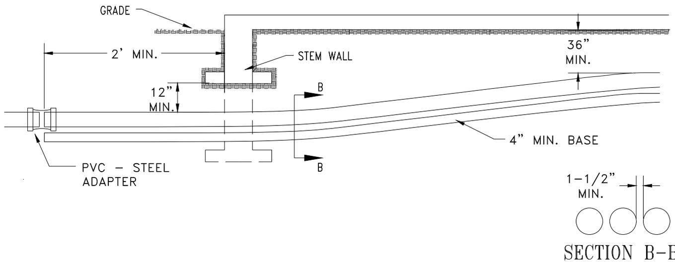
1. Conduits must be separated a minimum of 1-1/2".
