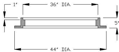
36" DIA. CAST IRON FRAME
