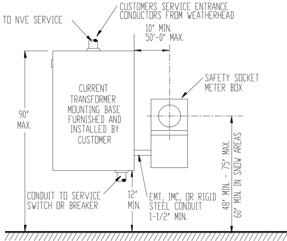
For single overhead irrigation service which is to be metered using current transformers, the customer shall furnish, install, own and maintain a separate current transformer cabinet and safety socket meter box and required service entrance conductors, conduit and weather head to the point of attachment of NVE's overhead service. The bussed current transformer cabinet is also acceptable for this application. Equipment shall conform to EUSER C Standards.
