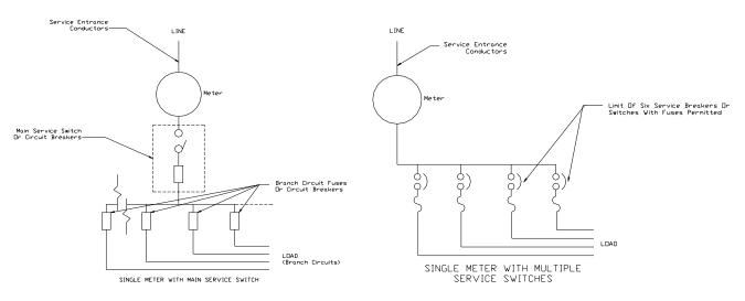
The meter switch may be located inside or outside the building being served in accordance with applicable electrical codes. Inside mounted disconnects will require the installation of a shunt trip device outside the premises.
