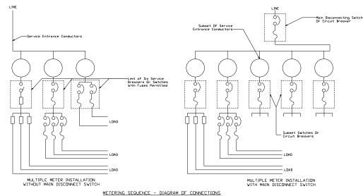
*For larger multi-meter installations (7+ meters) electrical codes require the installation of a main service switch or breaker located on the supply side of the meters.* In these instances, an individual meter switch must also be installed on the load side of each meter.
