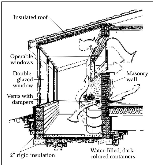
Sunspaces incorporate thermal mass to absorb solar heat. Solar-heated air can then be used to heat the house, either passively through openings in the common wall or by blowing through ductwork into other parts of the house.
